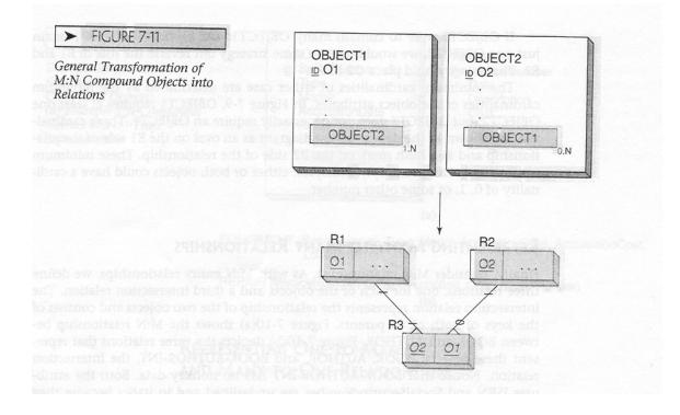
In general, for two objects that have an M:N relationship, we define a relationR1 for object OBJECT1, a relation R2 for object OBJECT2, and a relation R3 for the intersection relation. The general scheme is shown in **Figure 7-11**. Note that the attributes of R3 are only O1 and O2. For M:N compound objects R3 never contains nonkey data. The importance of this statement will become clear when we contrast M:N compound relationships with association relationships.
