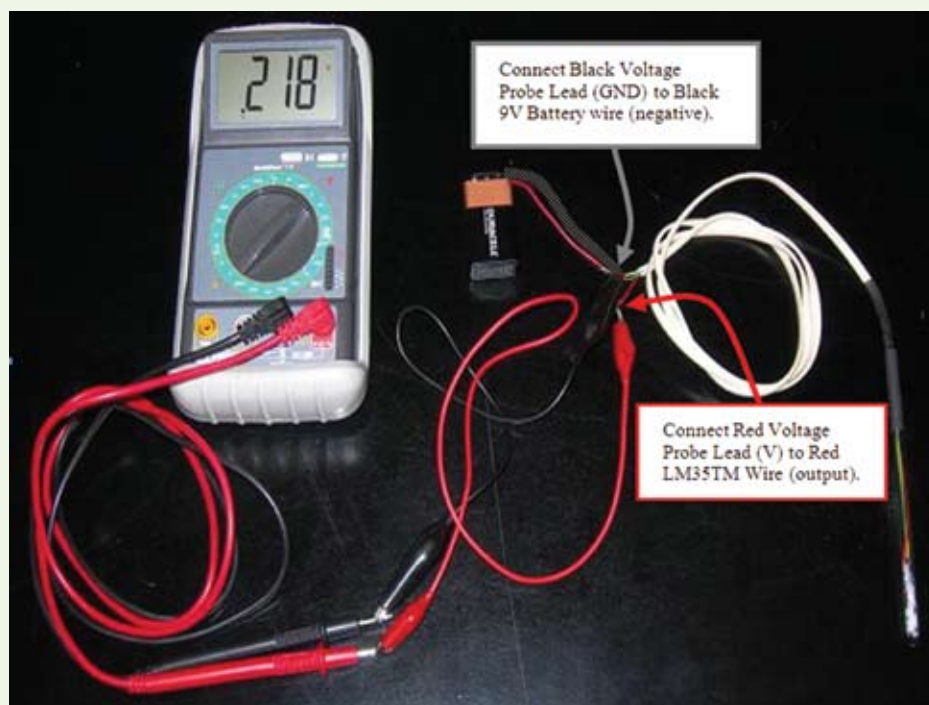
FIGURE 2 Digital thermometer with power supply (9V battery) and readout (digital voltmeter).
