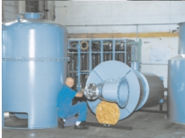
Deck water seal (semi-dry type) and pre-cooler unit
