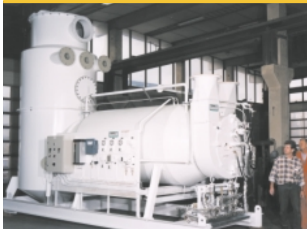
Generator unit of a 15,000 Nm 3 /h Flexinert system prior to delivery to a North Sea shuttle tanker
