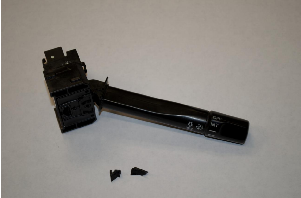
Figure 1: Windshield wiper switch as it sits in steering column. (Broken bits at the bottom)
