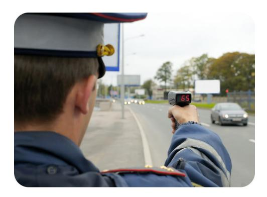
This police officer is pointing a gun at oncoming traffic. But it's not the type of gun that can be used as a weapon. It's a radar gun, and it's used to detect the speed of moving vehicles. Do you know how a radar gun works? Instead of shooting bullets, it "shoots" electromagnetic waves.
