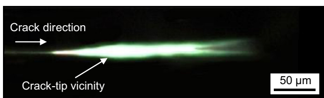
Fig. 6. Transmission optical micrograph from the (non-propagating) crack-tip region of the DN4PB test specimens showing the plane-stress region taken between crossed polarisers. For the anhydride-cured DGEBA epoxy polymer containing a v_f = 0.065 of silica nanoparticles.
