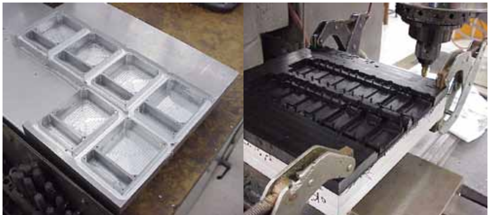
"Mass production" of PicoSat bodies (left) and battery bracket (right).
