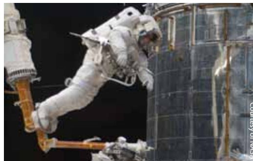
STS-125 astronauts navigate the exterior of the Hubble Space Telescope on the end of the remote manipulator system arm, controlled from inside Atlantis' crew cabin.
