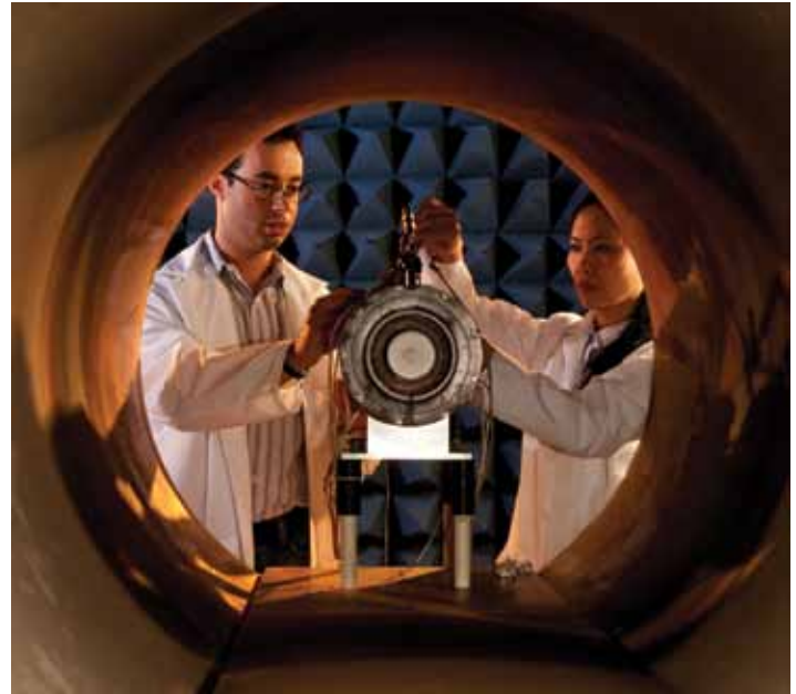
Rostislav Spektor and Xuan Eapen, senior research associate, investigate the origin of Hall thruster electromagnetic emission in the EMI facility.
