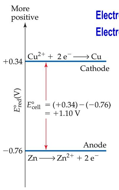
Electrode with more positive E° is cathode. Electrode with more negative E° is anode.
