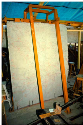
Figure 14. Monotonic load test to structural bahareque .
