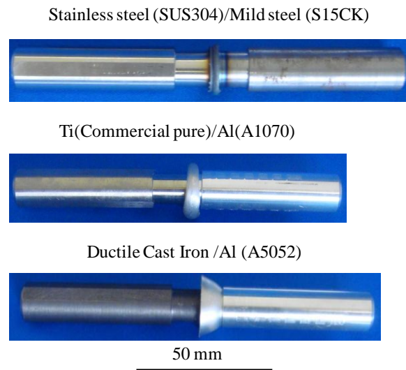
Figure 1. The pictures of the bimetallic specimens.
