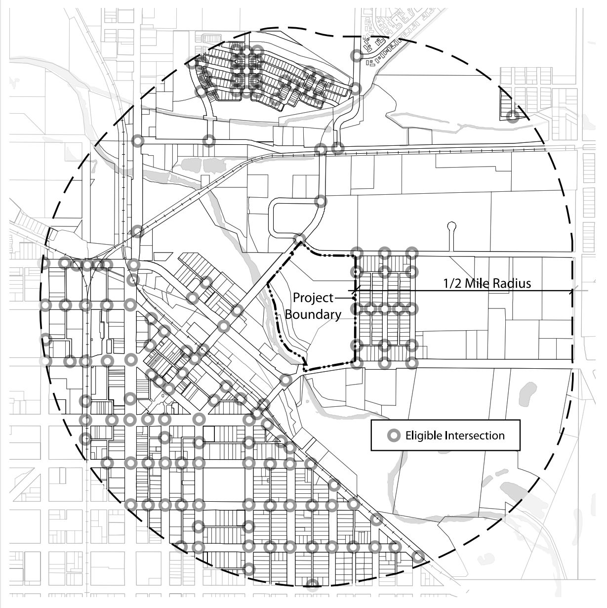
(d). Infill project site based on minimum 140 intersections/sq.mi. within 1/2 mile of project boundary
