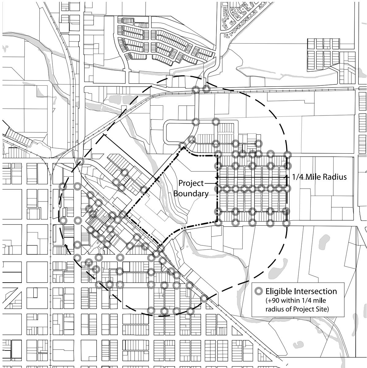
Figure 2. Project site with at least 90 eligible intersections per square mile within 1/4 mile of project boundary
