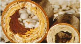
form of a more or less hard adherent crust. Such deposits are due to the fact the water loses its soluble power at high temperatures or because the concentrations become so high, due to evaporation, that the impurities crystallize and adhere to the boiler surfaces. The opportunity for the formation of scale in a boiler will be apparent when it is realized that during a months operation of a 100 horse power boiler , 300lbs of solid matter may be deposited from
