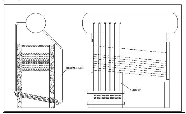
The illustration shows a boiler converted for FBC firing. In this boiler vibration of riser tubes was experienced. Even after a snubber support was provided, the vibration continued. The circulation calculation showed a velocity of 7 m/s in riser tubes. The vibration problem vanished after one of the risers was removed. The velocity in the riser was then estimated to be less than 6 m/s.
