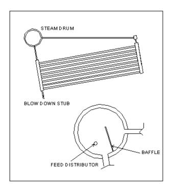
The bottom rows of the bank tubes of this cross tube boiler were sagging.
