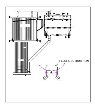
In this case, the water wall & bed coils were failing after bulging & overheating. Thick rough edge cracks were observed wherever the failure took place. There were several locations at which the failures had taken place.
