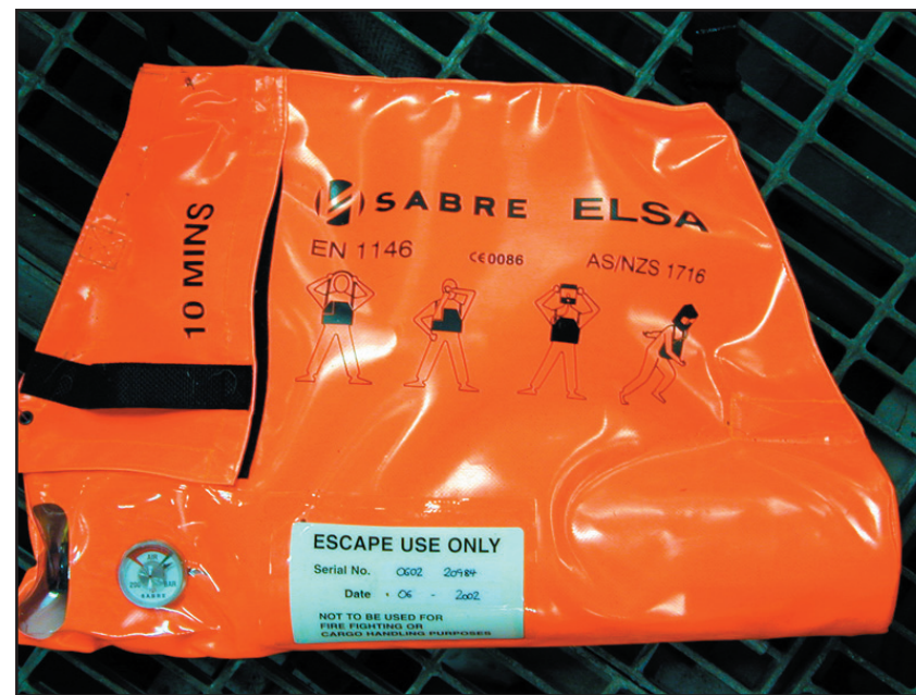
ELSA Situated In Engine Room
