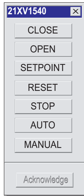
Control Valve Operation Menu
