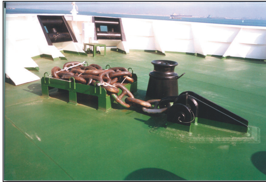
Forward Emergency Towing Chain
