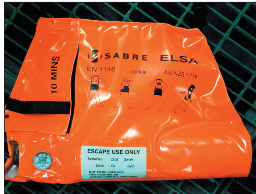
ELSA Situated In Engine Room
