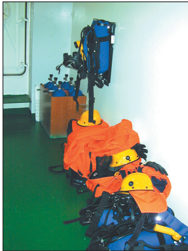
Breathing Apparatus Sets in Safety Equipment Locker
