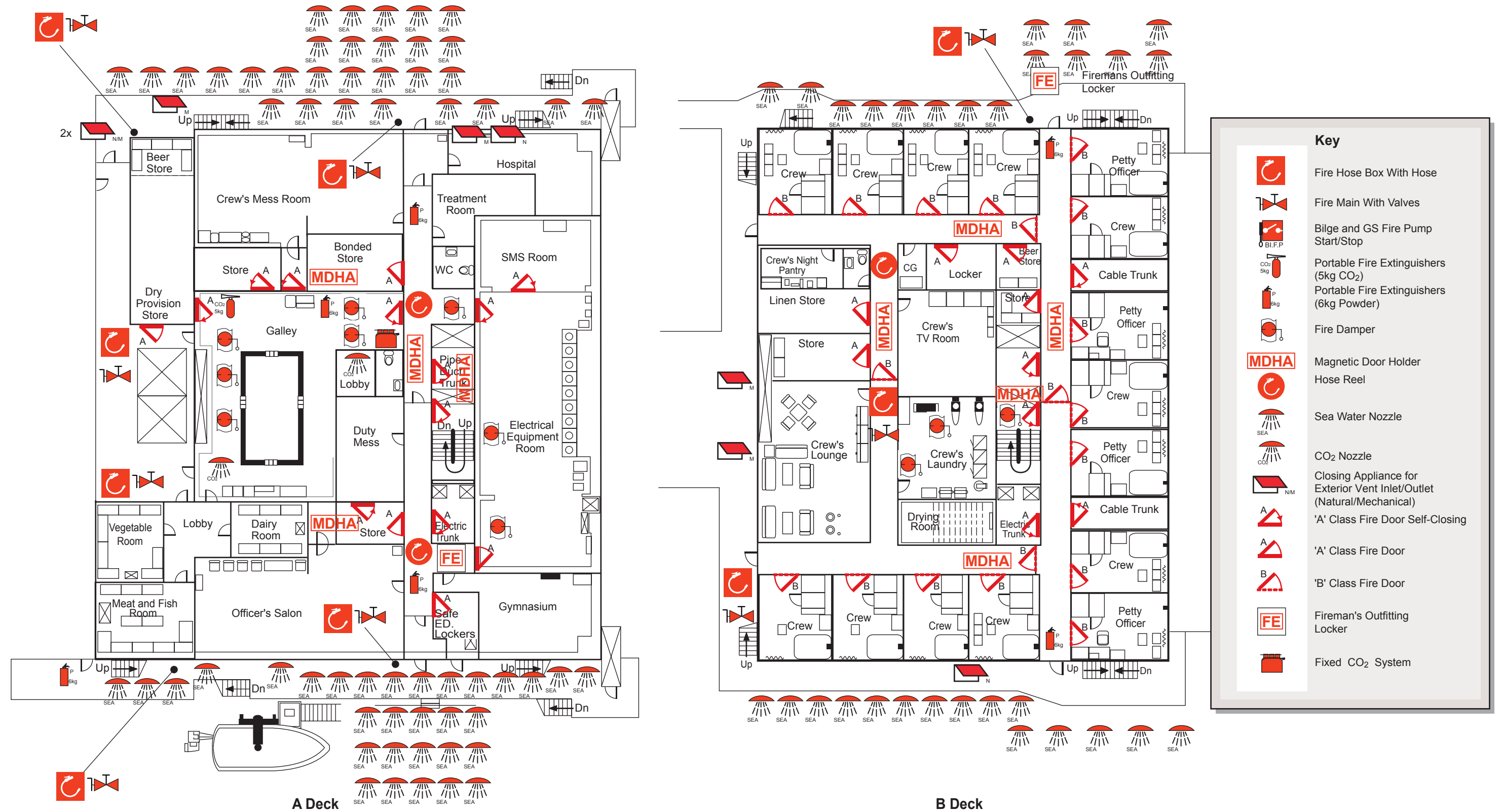
Illustration 3.4.8a (4) Fire Fighting Equipment on A and B Decks
