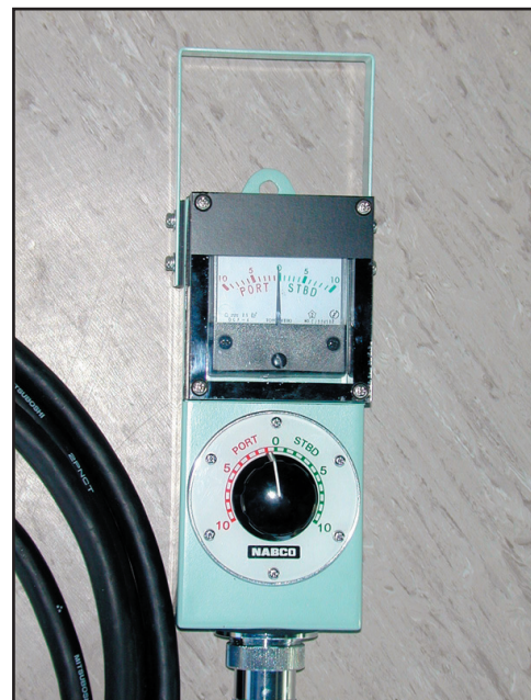
Bow Thruster Bridge Wing Control Unit
