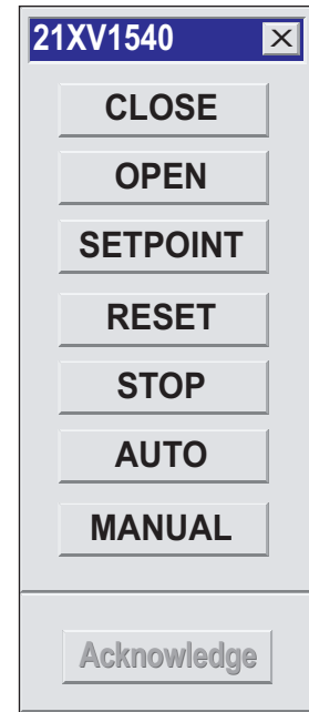
Control Valve Operation Menu
