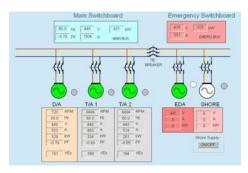
Power from the three main alternators, emergency alternator and shore supply is fed via Air Controlled Circuit Breakers (ACCBs). These have overcurrent, undervoltage and reverse power trip protection.
