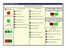
The second column shows the status of possible trip conditions that would either prevent the initial ignition sequence from proceeding or cause a boiler trip. These conditions are:
