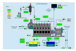
generator. The diesel engine is 4-stroke single acting turbo-charged, charge air-cooled trunk piston type engine. It is a self-contained unit with a wet LO sump and following engine mounted auxiliaries:
