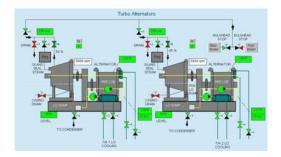
A pre-lubricating oil pump draws directly from the sump and discharges into the same lubrication manifold. The Pre-lube pump must be started before attempting to start the turbine. However the mechanical pump provides lubrication as the turbine rises to operational speed at which point the pre-lube pump can be shut down.
