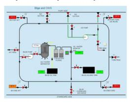
The bilge pump system can be set to automatic. Cross connections between the general service pumps and the fire pump are also available
