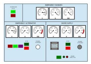
The emergency switchboard monitors the emergency busbar conditions and is equipped with meters for Voltage (V), Current (kA) and Real Power (kW). It also supports controls for the tiebreaker ACCB
