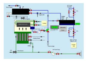
Fresh water is discharged through a distillate pump and directed by a three 3 way control valve either to storage or, if the salinity is high, to the bilge system. Fresh water is stored in either (or both) the Shore Supply Fresh Water Tank or Distilled Water Tank. Brine ejection is assisted by the flow of seawater generated by the SW Feed Pump.
