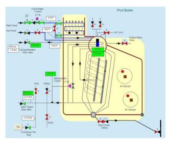
The boiler is fitted with two fuel oil and two gas burners. The fuel burner is assisted by atomizer steam and has a forced draught air register and fuel oil shut off valve. Fuel is distributed to the burners from separate gas and oil burner manifolds. The operation of increasing or decreasing the number of burners can be manual or automatic.
