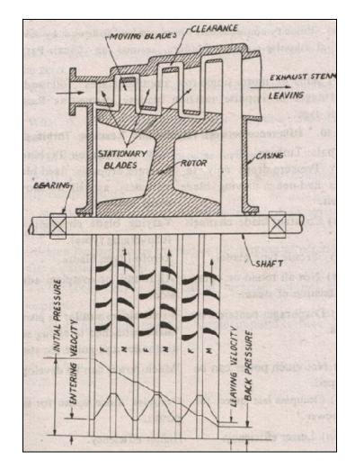
Differences between Impulse and Reaction turbines
