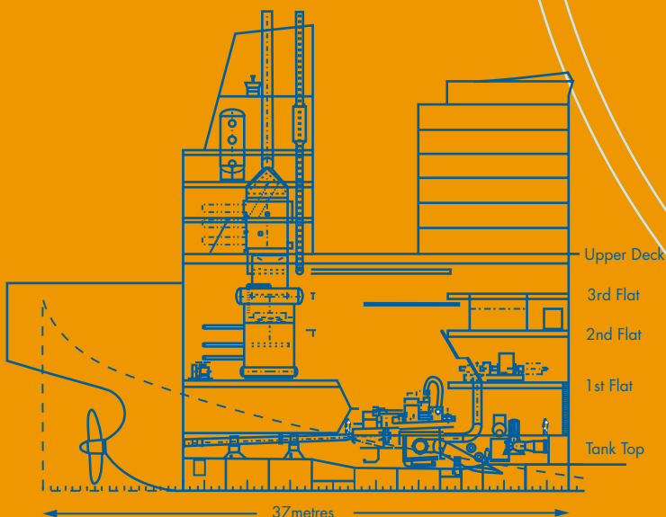
A TYPICAL STEAM TURBINE PROPULSION SYSTEM
