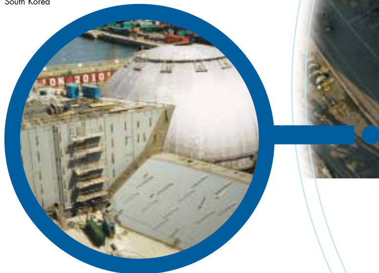
Free-standing Moss ship under construction at Hyundai Heavy Industries, South Korea
