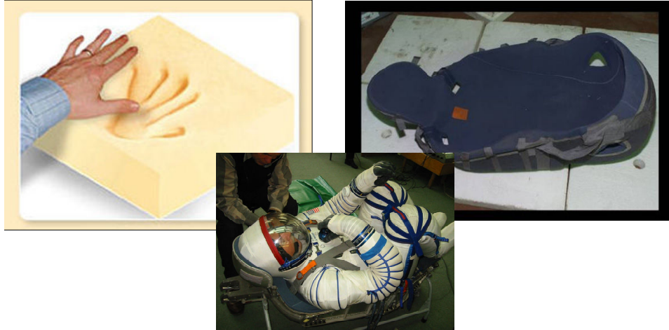
Figure 17. Two-layer foam seat-liner design composed of an outer non-Newtonian fluid and an inner layer of memory foam.
