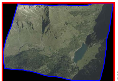
Figure 9 – footprint and bounding box of an orthoimage (respectively in blue and red)
