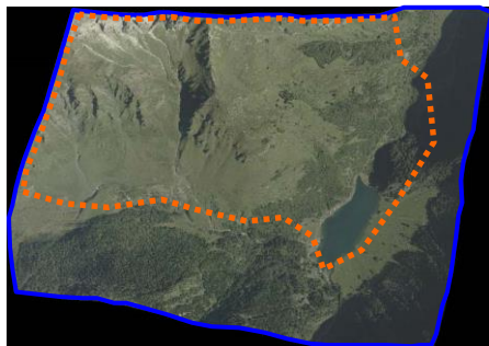
Figure 11 – footprint and contributing footprint of an orthoimage referred by an aggregated orthoimage (respectively in blue and orange)
