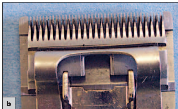
16.3 With repeated sharpening, the distance between the tips of the clipper guard and cutting blades reduces. The blades in (a) have been sharpened too many times and the tips of each blade are so close together that trauma to the skin is likely. In (b) there is still an appropriate gap between the two rows of tips.
