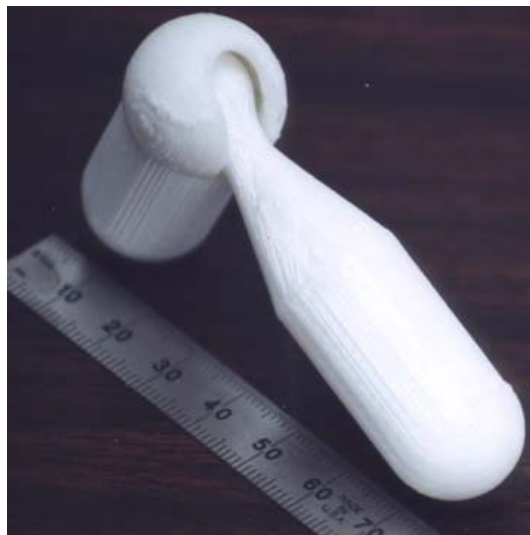
Figure 2: Functional Ball Joint made via FDM
