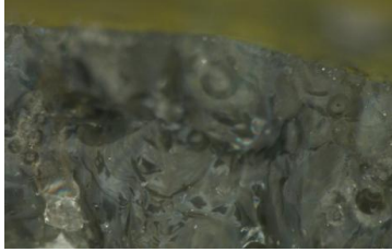
Figure 2: Transparent glass created with SLM
