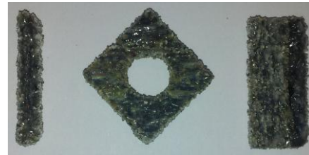
Figure 1: Sample parts created by SLM from sand
