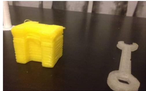
Figure 5: Two Parts Printed in Microgravity; a Standard ESAMM Coupon and a Wrench
