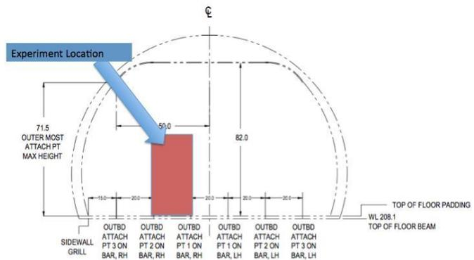
Figure 2: Location of Experiment Inside Aircraft
