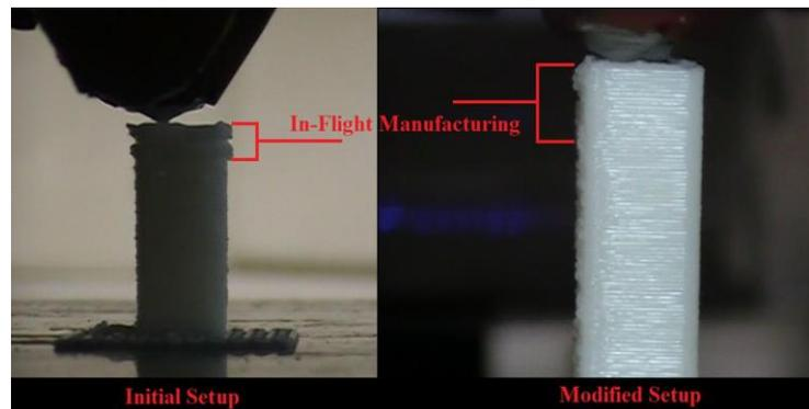
Figure 6: In Flight 3D Printed Part Before and After Modification
