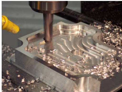
Figure 1. Milling: a subtractive manufacturing process [2].
