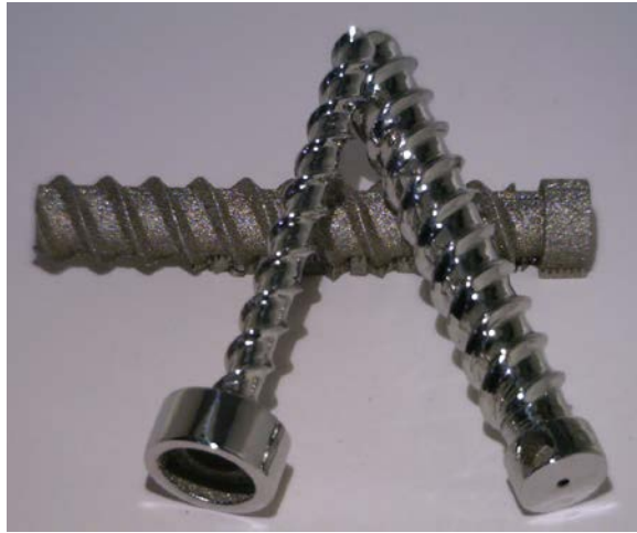
Figure 13. Powder bed fusion bolts with finished and unfinished surfaces [20].
