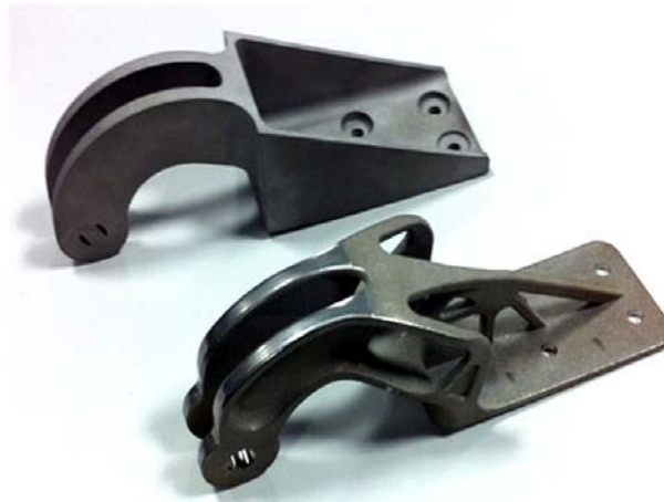
Figure 19. The background hinge was produced using conventional subtractive manufacturing techniques. The hinge in the foreground was produced using additive manufacturing techniques and is half the weight. The hinges were produced by EADS [36].
