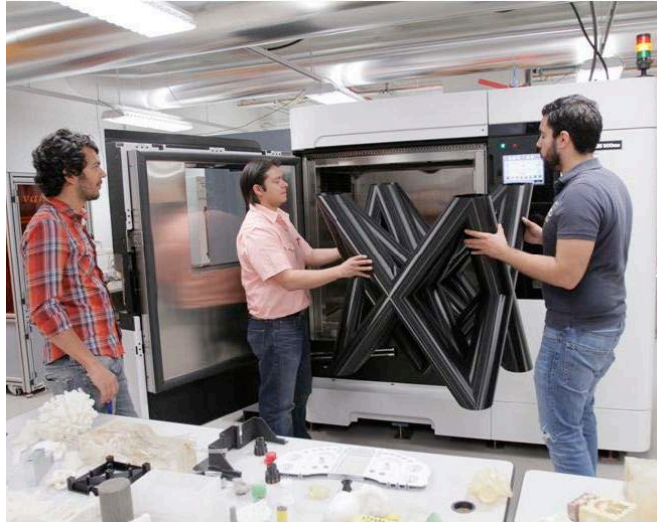
Figure 9. Stratasys Fortus printer showing the large 3' x 2' x 3' build volume (picture taken at UTEP, courtesy of Francisco Medina).
