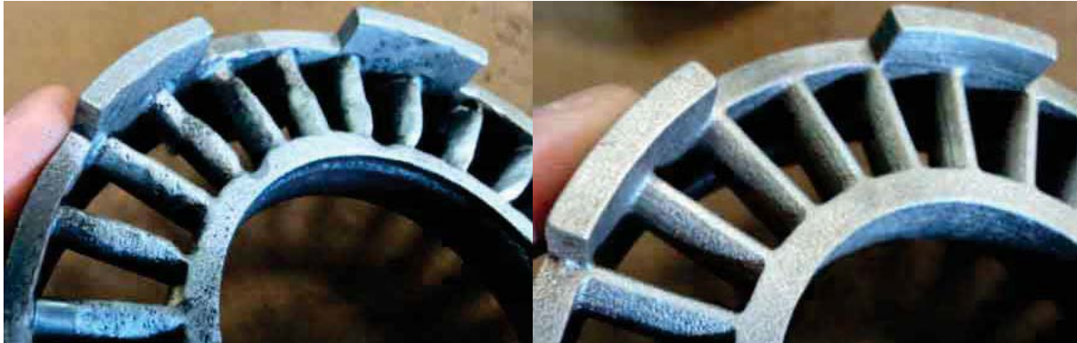
Figure 5. From left: wear in conventionally machined 4145 steel stator after 200-300 hours; 3D printed part showing no measurable wear after 600 hours [6].
