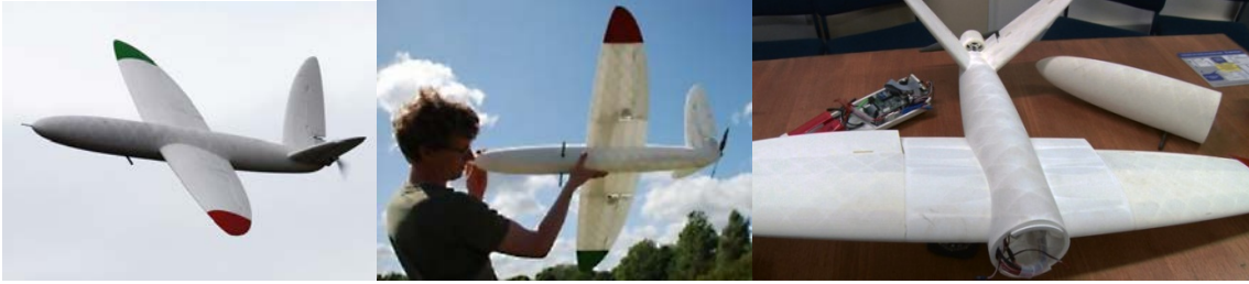
Figure 14. SULSA is the world's first "printed" aircraft. The University of Southampton printed the UAV structure allowing the entire vehicle to be assembled in about 10 minutes without tools [24, 25].
