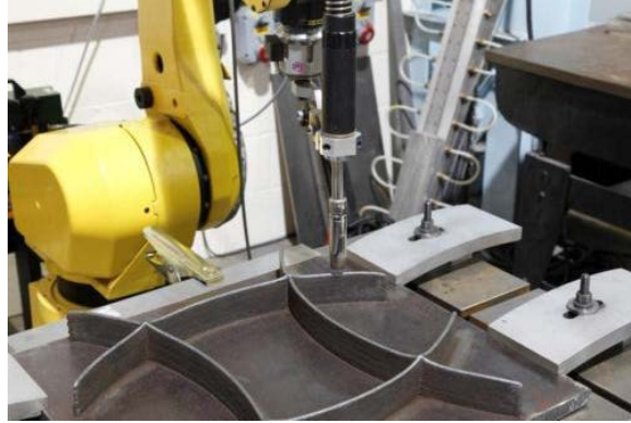
Figure 7. Canfield University gas metal arc welding robot depositing material [13].
