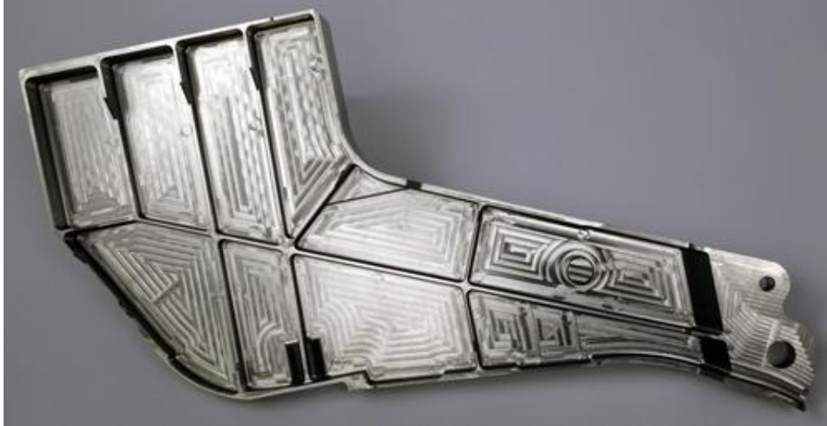
Figure 6. Ti component made by Sciaky for potential use in the Joint Strike Fighter (JSF) program [10].
