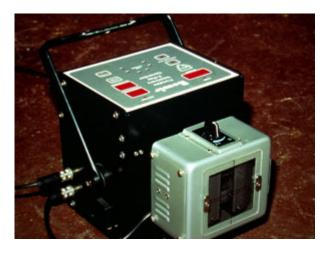
This is a typical portable x-ray unit produced for equine practitioners. This unit is capable of 10 mA and 80 kVp so is suitable only for the distal limbs.
