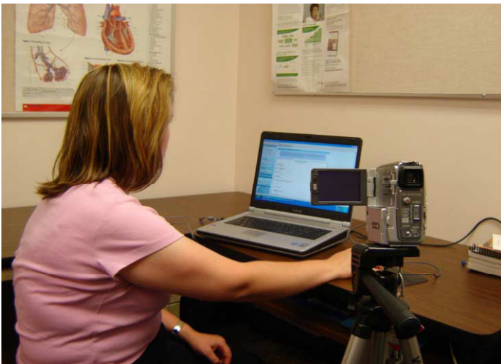
Figure 3. Example of low-cost rapid usability engineering set up for video recording health professionals as they work.
