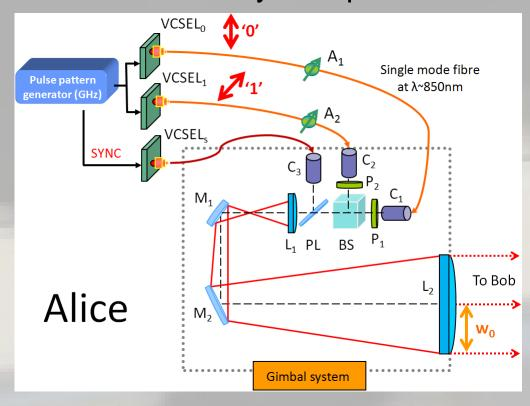
$A_1$  and  $A_2$  are fibre-coupled attenuators;  $P_1$  and  $P_2$  are high-extinction ratio polarizers;  $C_1$ ,  $C_2$  and  $C_3$  are optical collimators, BS is a 50/50 beamsplitter, PL is a pellicle beamsplitter;  $L_1$  and  $L_2$  are achromatic doublet lenses and  $M_1$  and  $M_2$  are high-reflectivity mirrors.
