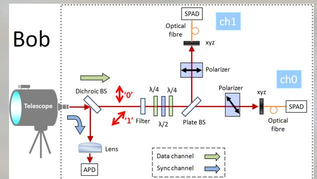
APD is avalanche photodiode; SPAD is single photon avalanche detector and xyz are traslation stages.
